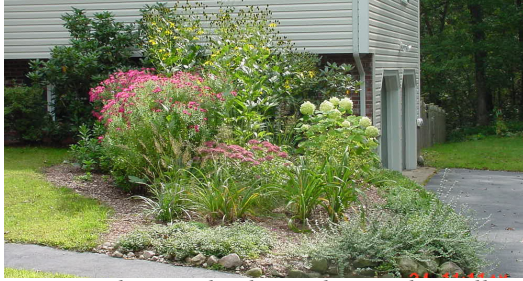
Rain gardens are landscaped areas that collect and treat stormwater runoff using bioretention.
