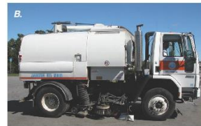
Figure 4. A, Pelican Series P mechanical sweeper and B, Johnston 695 Series vacuum sweeper, used in the evaluation of sweeper efficiencies.
